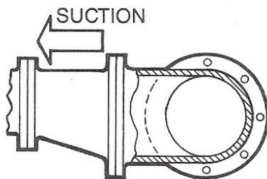
Avoid the use of valves and strainers in the suction line. Start up strainers must be removed shortly after start up. When the pump is installed below the source of supply, a valve should be installed in the suction line to isolate the pump and to permit pump inspection and maintenance. However, never place a valve directly on the suction nozzle of the pump.
