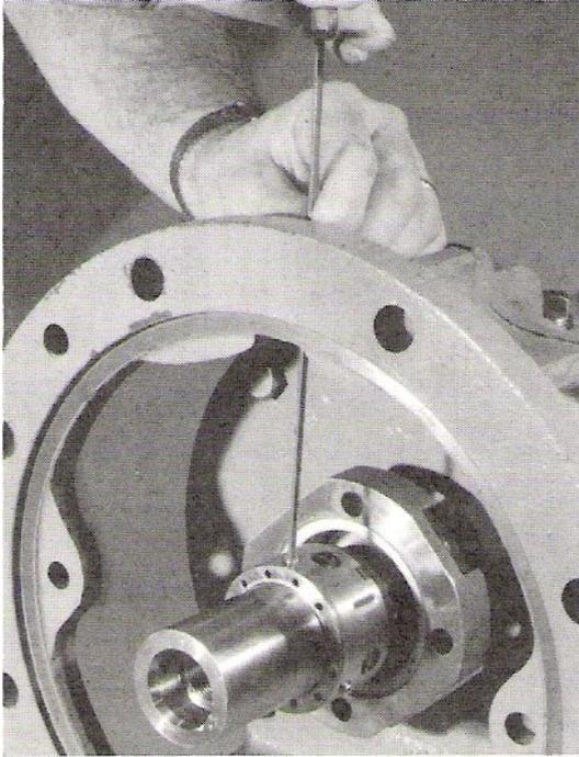
17. If a component type outside mechanical seal is used, remove the gland and the stationary seat. Remove the stationary seat from the gland. Loosen the set screws in the rotating unit and remove it. Discard all O-rings and gaskets.
