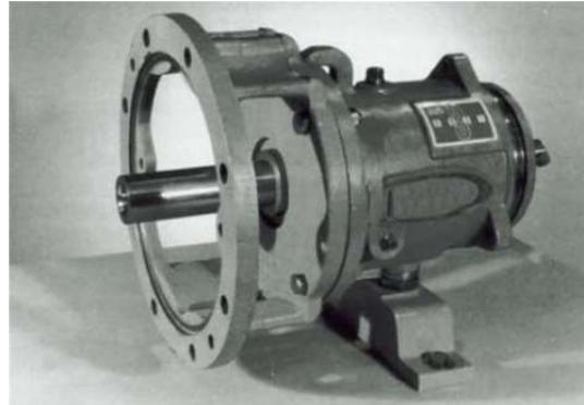
20. If the power end is oil lubricated, remove the drain plug (#134) and drain the oil from the bearing housing (#119).
