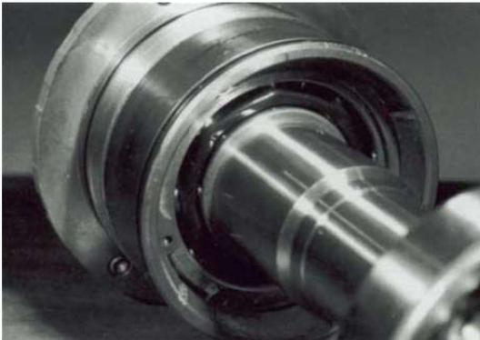
**Note:** Type 1 and 2 pumps equipped with duplex angular contact bearings use a bearing retainer (#201) instead of the snap ring. Remove the carrier from bearing.
