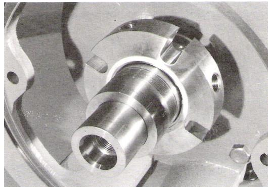
16. If a component type inside mechanical seal (#153) is used, loosen the set screws on the rotating unit and remove it from the shaft, see Figure 5-2. Then pull the gland (#190) and stationary seat off the shaft. Remove the stationary seat from the gland. Discard all O-rings and gaskets.
