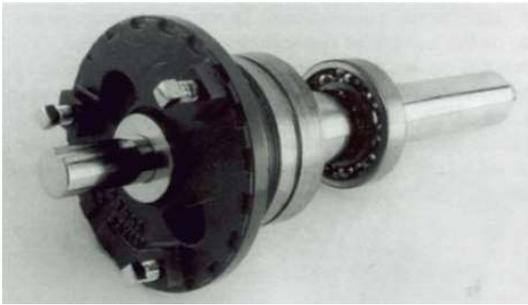
24. Remove the snap ring (#201C) (Figure 5-7) on Type 1 and 2 pumps, or the bearing retainer (#201D) on Type 3 pumps.
