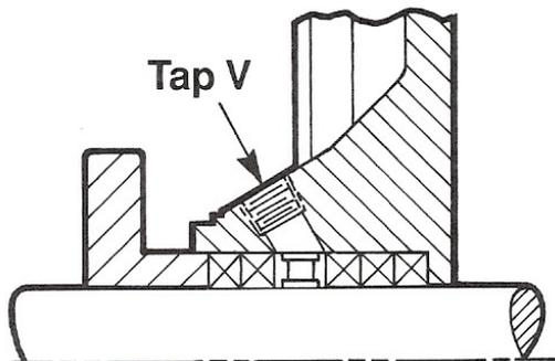
Grease lubrication, when compatible with the pumpage, may be used. In non-abrasive applications the pumpage itself may be sufficient to lubricate the packing. Again, introduced into Tap V.
